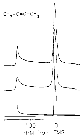
Figure 1. Carbon-13 spectra of 2-butyne: experimental, theoretical convoluted, and theoretical powder spectra are shown from top to bottom.
